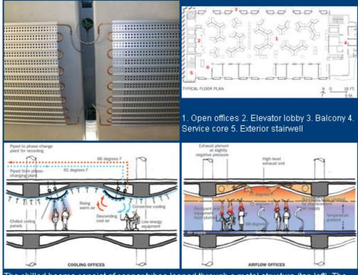
The chilled beams consist of copper tubes looped through a metal structure (top left). The tubes tie into chilled water supply and return lines running in the cavities behind the precast-concrete panels. The slot between the panels is also used for lighting cabling. In passive mode, fresh air is supplied from the floor only (bottom right). In active mode, the chilled beams operate and cool down the air supplied from the floor (bottom left). Photos © Russell Fortmeyer
