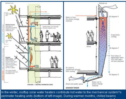
In the winter, rooftop solar water heaters contribute hot water to the mechanical system?s perimeter heating units (bottom of left image). During warmer months, chilled beams integrated into perimeter light shelves cut down on heat gain from sunlight (top of left image). On the south side of the building, five ?shower towers? provide additional cooling to water for the mechanical system (right).
