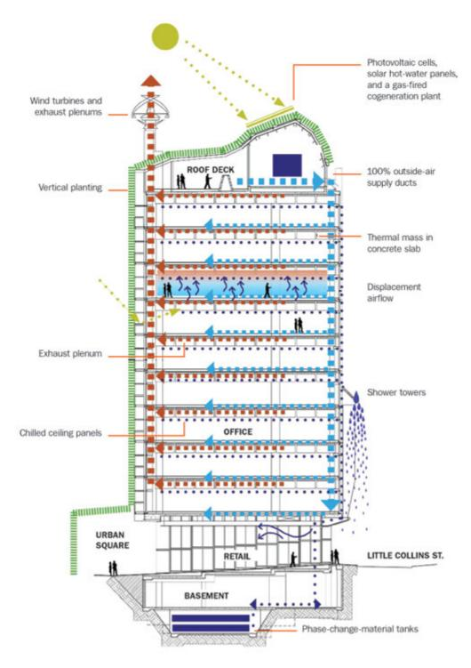
As the sun drifts west, the timber panels slowly close. The phase-change-material tanks in the basement are part of the comprehensive HVAC strategy for the CH2 building.
